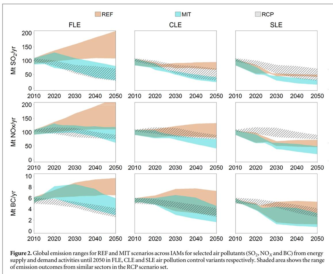
**Figure 2.** Global emission ranges for REF and MIT scenarios across IAMs for selected air pollutants (SO<sub>2</sub>, NO<sub>x</sub> and BC) from energy supply and demand activities until 2050 in FLE, CLE and SLE air pollution control variants respectively. Shaded area shows the range of emission outcomes from similar sectors in the RCP scenario set.
