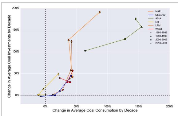
Figure 4. Decadal changes of average coal consumption in the electricity sector (*x*-axis) and average investment in coal-fired generation capacity (*y*-axis) for different regions (region categorization RC5 as defined in the IPCC AR5 [25]). Data source: [28, 35]. Note: please see figures S2 and S3 for annual changes.
