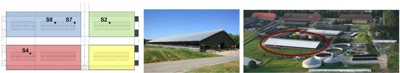
Fig. 1 – Description of the measurement site Dummerstorf: Layout of the barn (north front at the top of the map) and sensor positions (left), photography of the barn viewed from the main prevailing wind direction (middle, source: ATB) and a map of the farm indicating the position and orientation of the barn (right, source: Homepage Gut Dummerstorf).
