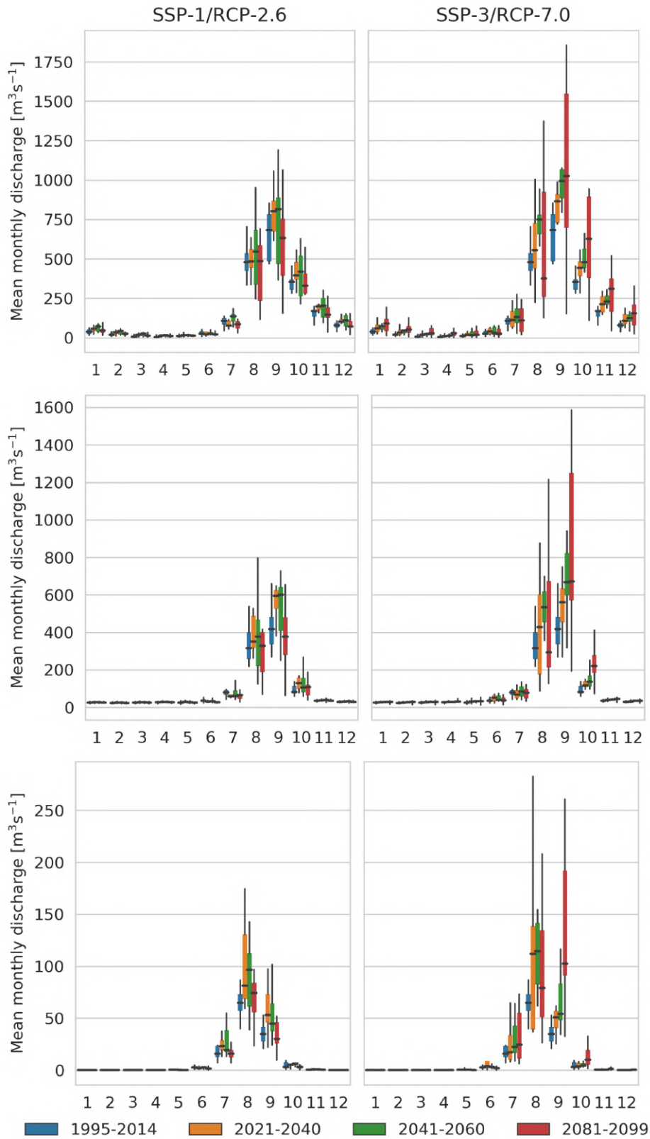
Figure 24: Mean monthly discharge in the reference period (blue) and the three future periods for SSP1-RCP2.6 (left) and SSP3-RCP7.0 (right) at Dapola (Black Volta, top), Yarugu (White Volta, middle) and Bge Yalogo (upper Sirba River, bottom). Error bars refer to the interquartile range (coloured) and the full ensemble range (whiskers).
