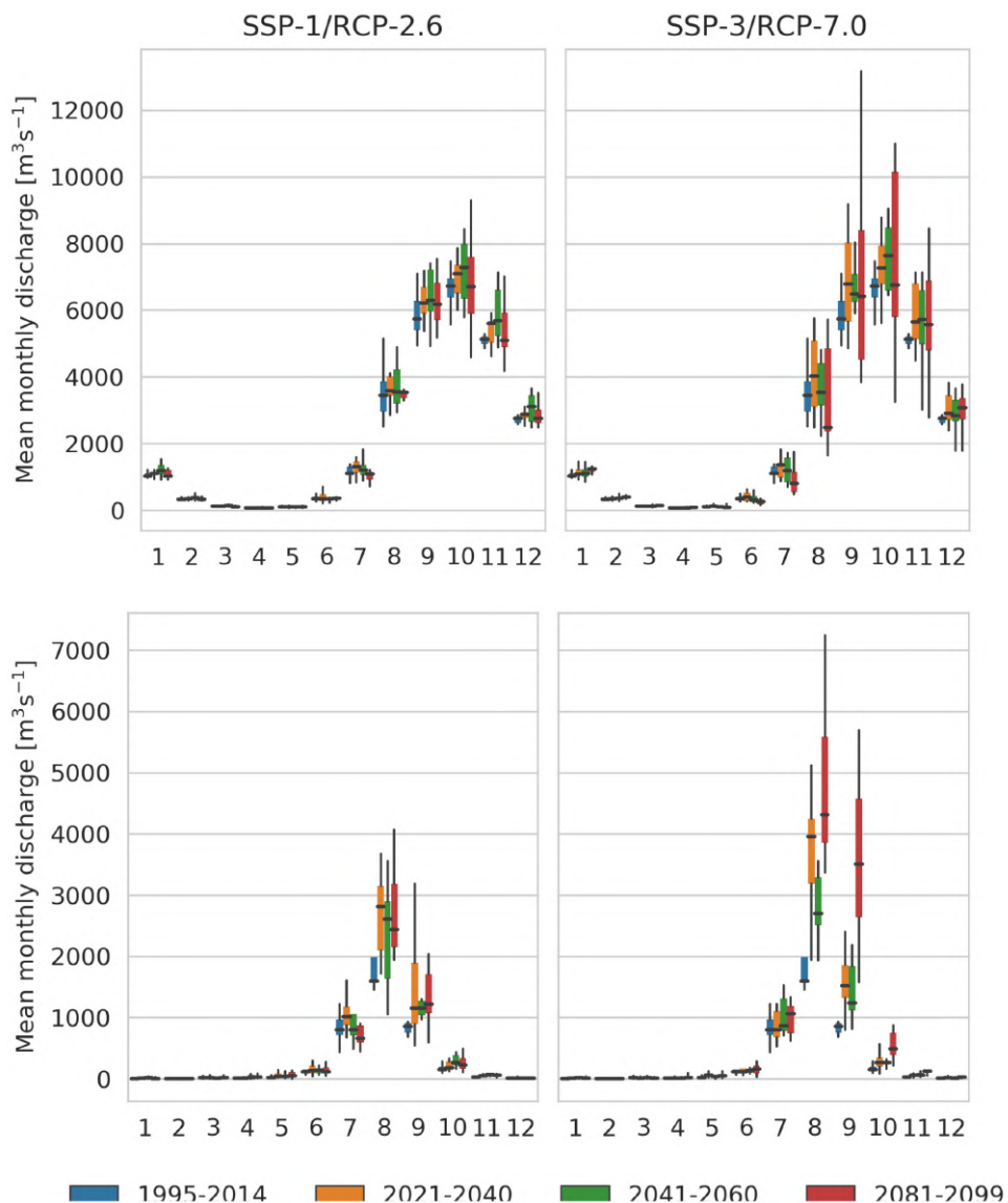
Figure 25: Mean monthly discharge in the reference period (blue) and the three future periods for the low emissions scenario (left) and the high emissions scenario (right) at Niamey (Niger River, top) and at Baleyara (Dallol Bosso, bottom). Error bars refer to the interquartile range (coloured) and the full ensemble range (whiskers).
