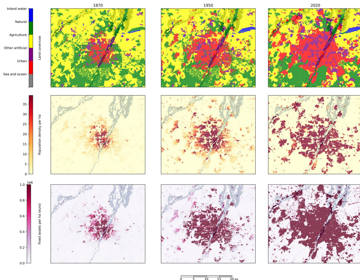
Fig. 10 An example of modelled exposure growth in the vicinity of Munich (NUTS region DE212), southern Germany, between 1870 and 2020, contrasted with a 100-year river flood map (grey shading). Flood hazard zone from Alfieri et al. 57 .
