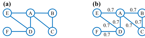
Fig. 1. An example of computing the expected degree of node A , the expected number of triangles, and the expected number of non-closed wedges associated with A . (a) The given graph \mathcal{G} . The degree of A , the number of triangles, and the number of non-closed wedges associated with A , are m_2^A(\mathcal{G}) = 4 , m_3^A(\mathcal{G}) = 2 (i.e., \{\{A, E\}, \{A, D\}, \{E, D\}\} and \{\{A, B\}, \{A, C\}, \{B, C\}\} ), and m_w^A(\mathcal{G}) = 4 (i.e., \{\{A, E\}, \{A, C\}\}, \{\{A, E\}, \{A, B\}\}, \{\{A, D\}, \{A, C\}\} , and \{\{A, D\}, \{A, B\}\} ), respectively. (b) The given graph \mathcal{G} with a uniform and independent sampling probability p = 0.7 . Based on Eqs. (2a), (2b), and (2c), the expected degree of A , the expected number of triangles, and the expected number of non-closed wedges associated with A , are \mathbb{E}_2^A = 2.8 , \mathbb{E}_3^A = 0.686 , and \mathbb{E}_w^A = 2.254 , respectively.
