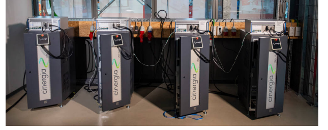
Fig. 4: Four inverters in the power hardware in the loop lab. While structurally similar, the implemented control differs significantly from the EMT model.
